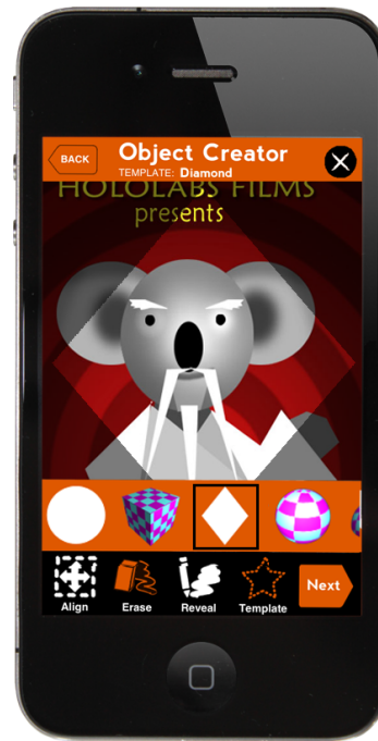
Figure 4: Screenshot of the Farrago Object Creator, showing how textures are mapped onto template objects.
